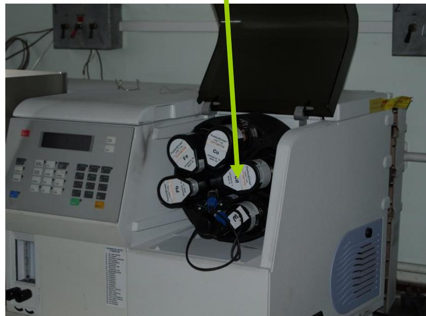
Figure 12.9 - a hollow cathode lamp located within AAS instrument
