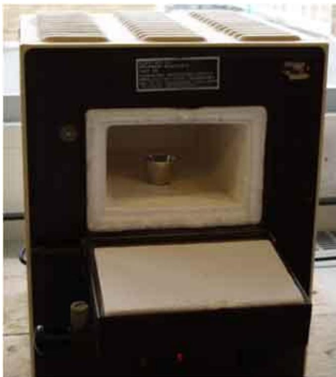
Figure 12.2 - a typical small muffle furnace used for dry ashing (sample containing crucible located inside the furnace)
