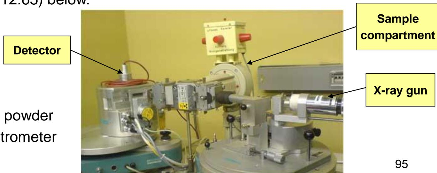
Figure 12.65 – powder diffraction spectrometer
