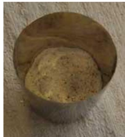
Figure 12.3 - a crucible containing a sample for dry ashing
