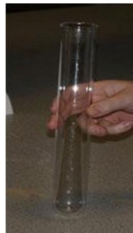
Figure 12.46 - glass digestion vessel.
